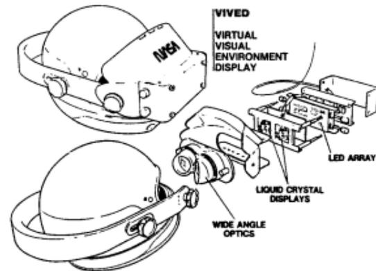
Fig. 1. HMD of Nasa's Virtual Visual Environment Display (VIVED) project.
